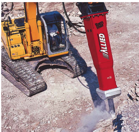
The m14 requires a hydraulic flow of 48 gpm at 2,320 psi and breaks at the rate of 1,000 bpm. The m18 needs 58 gpm at 2,320 psi and delivers 800 bpm. The hammers have working weights of 3,042 and 4,145 pounds, respectively. Recommended carrier weights for the m14 range from 40,000 to 53,000 pounds, and from 46,000 to 71,000 for the m18.
