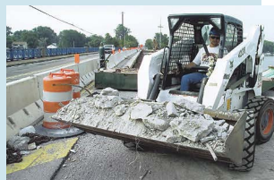
The Bobcat A300 features a 3,000-pound rated operating capacity and 126.4-inch lift height. It comes with a 20.7-gpm standard flow auxiliary hydraulic system.
