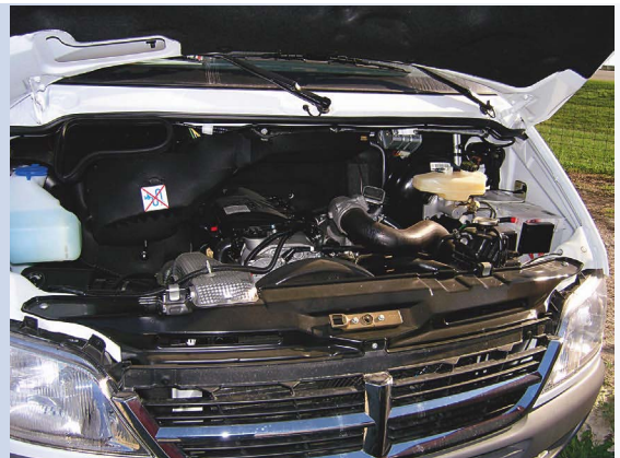
Left: Among loyal customers, Ram's Cummins I-6 Turbodiesel is a legend in its own time, and the latest version is both clean and quiet. Sprinter's small I-5 Mercedes Turbo Diesel is fast off the line and claims great fuel economy.
