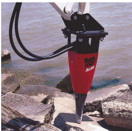
Rammer in-Series models, which range in weight between 152 and 453 pounds, and deliver between 1,800 and 2,100 bpm, require hydraulic flows ranging from 8 to 18 gpm and operating pressures from 2,030 to 2,175 psi. List prices range from $4,950 to $8,750.
