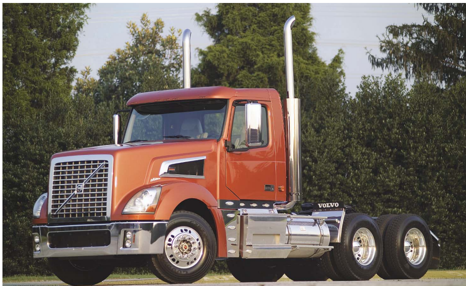
VT 800 features bold styling and a big hood to house Volvo's D16 or Cummins' ISX diesels, with cooling to handle their high horsepower. The new model is built to pull heavily loaded lowboys and equipment trailers, as well as other duties requiring Big Power.
