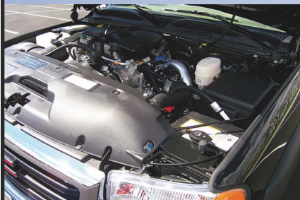
The Duramax 6600 now has 310 horsepower with torque of 605 lbs.-ft., but a new version due out about now will have 360 horsepower and 650 lbs.-ft. — the strongest pickup engine available, unless competitors up the ante.
