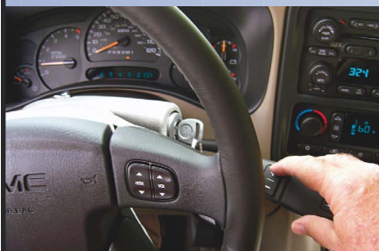
A Tap Shift switch on the selector lever allows easy up- and downshifts, while digital readout on dash tells which gear the Allison's in.
